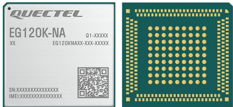
Figure 49: Top and Bottom Views of EG120K-NA
